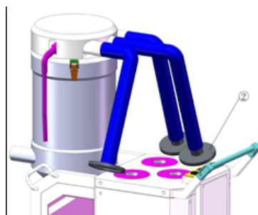
Step 2: Remove the filter lid from the top lid.
